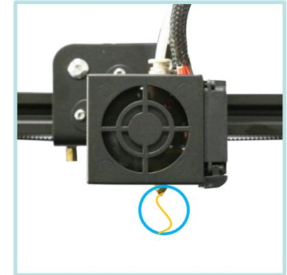
Press and hold the extruder lever then insert 1.75mm filament through the small hole of the extruder. Continue feeding until you see filament come out the nozzle.
