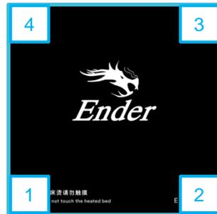
3. Move the nozzle the front/left leveling screw and adjust the platform height by turning the knob underneath. Use a piece of A4 paper (standard printer paper) to assist with the adjustment, making sure that the nozzle lightly scratches the paper.
