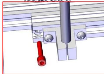
**i** Note: Align the bottom profile, then tighten the screws.
