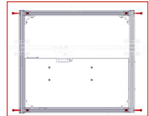
**i** Note: Tighten the four screws on the top, then tight the side screws.
